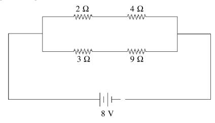
9) A multiloop circuit is shown in the figure. It is not necessary to solve the entire circuit. Determine the current  $I_2$ .
